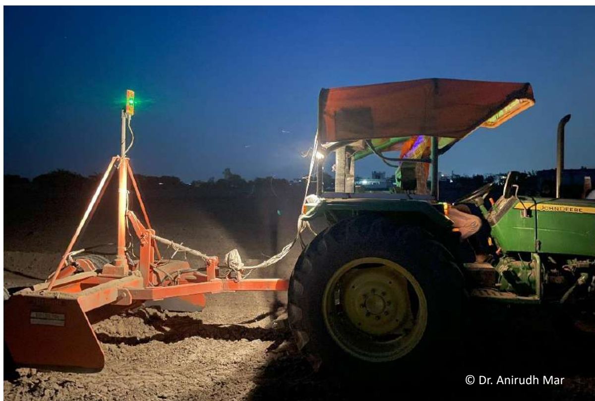
Laser land levelling technology operated at night in northwest India.
