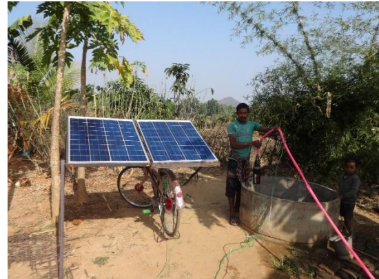
Cycle Mounted Solar Pump connected with drip irrigation system of Tata Trust – an auxiliary technology
